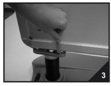
3. Frame can be lift off easily with a special key that is part of the package.
